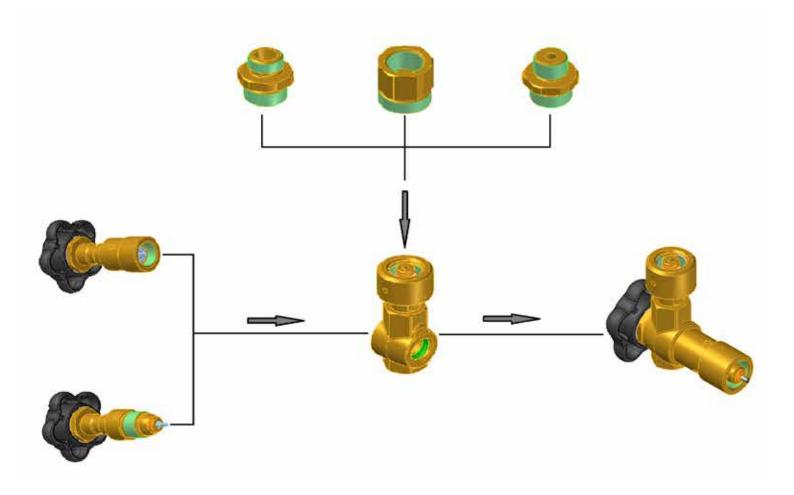
Only use the MGE recommended O-ring for the different gas types to ensure compatibilty.
